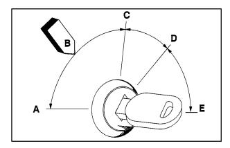
With the ignition key in the ignition switch, you can turn the switch to five positions.
